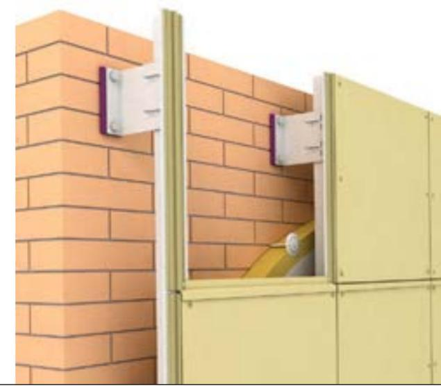
Fiber cement is a composite building material composed of cement, quartz sand, cellulose fibers and water. The cellulose fibers in the composition act as a reinforcing agent, that is, they give the required strength to the material.
